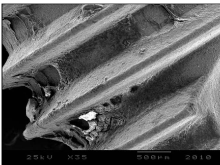
Fig. 5. SEM of the cervical and middle thirds of the failed ART screw type implant after 7 weeks of insertion, showing peeling off of some of the implant coating at the implants surface (25 kV, magnification, \times 35 ).
