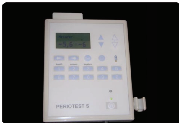
Fig. (6) Periotest S device readings during measuring implant stability
