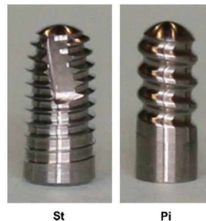
Fig. 1. Representation of implant designs used in this study: Screw type (St, left) and Push-in (Pi, right).
