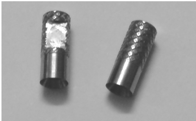
Fig. (4): Laboratory implant analogues.
